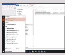
Expand the 'Ports (COM & LPT) list. The Actisense USB device will be displayed with '(COM X)' (X refers to the COM Port number) next to it.
