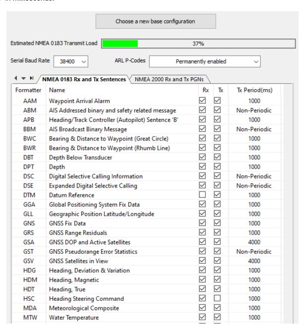
Once the various configuration options have been configured as required, the "Estimated NMEA 0183 Transmit Load" bar will indicate whether the configuration will work as expected (when the load is 100% or below) or whether the transmit rates in reality may be lower than requested (when the load is above 100%) due to output overload.
