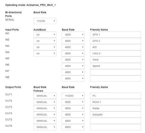
From this point onwards, the Friendly names entered in the previous page for the baud rate configuration will prove very useful in setting up the rest of the steps on the current user mode, because they carry through.
