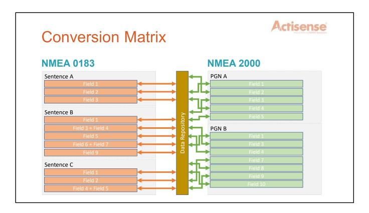
As the inner workings of NMEA 2000 Gateways vary from manufacturer to manufacturer, this last section will need to focus on how the Actisense NGW-1 and W2K-1 perform their NMEA Conversions.
