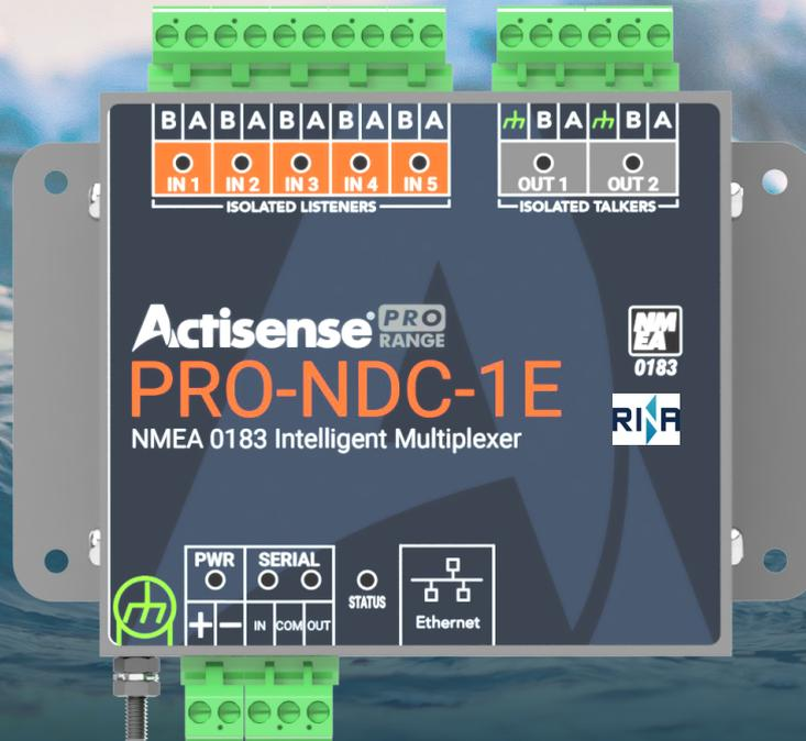
The PRO-NDC-1E is a RINA type-approved intelligent NMEA multiplexer, housed in a rugged stainless steel enclosure which provides isolation on all inputs and outputs.
