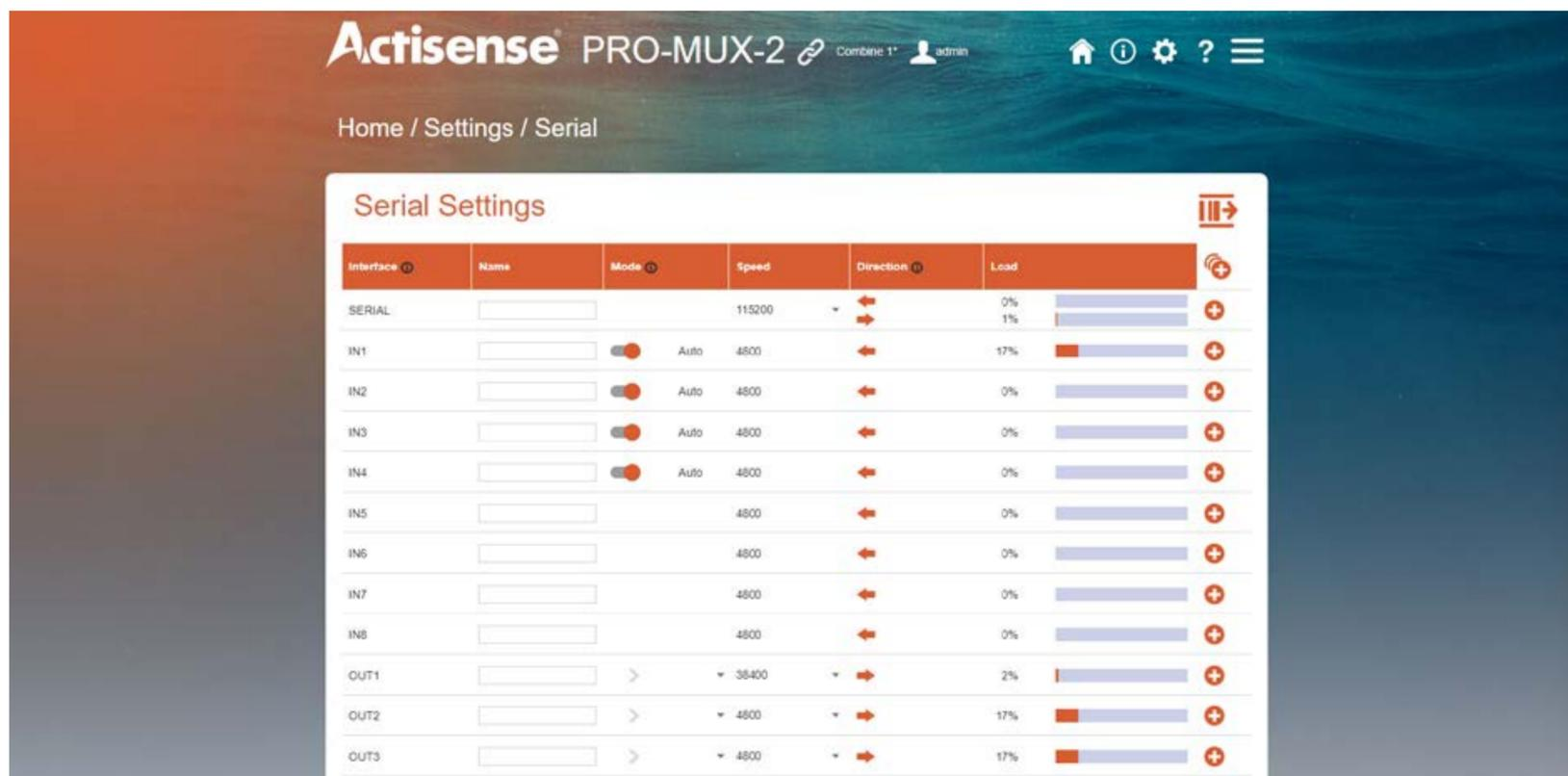
The serial settings are where the baud rate is individually configurable for each input port and output port, and a 'friendly name' can be given to each port. There are two routes that can be taken here for talker devices connected to the inputs:
