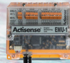
EMU-1 NMEA 2000 Engine Monitoring Unit
