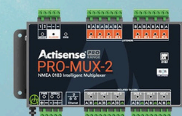
PRO-MUX-2 NMEA 0183 Intelligent Multiplexer
