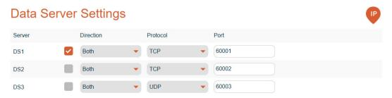
If you are only using the W2K-1 to send data to OpenCPN, then the direction can be set to 'Transmit Only.' However, if you also want OpenCPN to send data such as waypoints back to the W2K-1, then set the direction to 'Both.'
