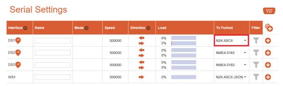
The Data direction is dependent on what you are using the W2K-1 with OpenCPN for, but this can be changed under Settings > Data Server:
