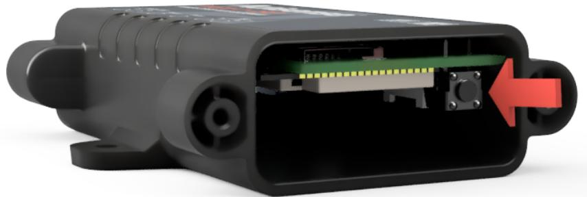
Carefully power the device up ensuring that there is no chance of anything touching the PCB which could cause shorts and damage the device. Depress the pushbutton for 5 seconds, then release it. The device should restart after a further 5 seconds with the passwords reset to default.
