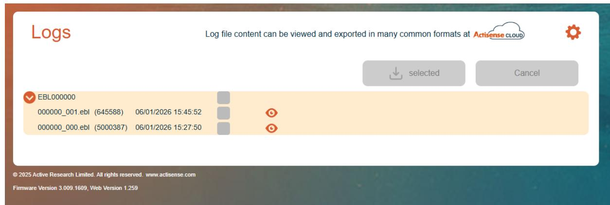
The length of time before the SD card becomes full depends on the amount of data on the NMEA 2000 network. When the SD card is full, it will begin to write over existing log files, starting with the oldest.
