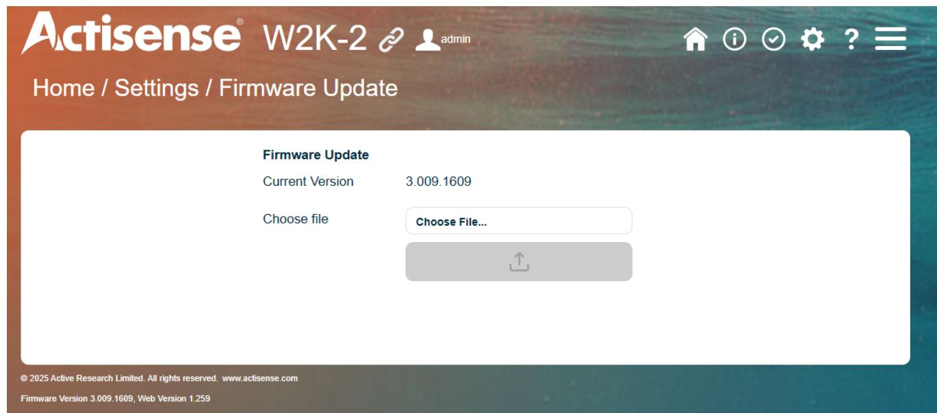
**Note:** Do NOT extract files prior to upload. Firmware updates in the correct '.zip' file format for the W2K-2 are available from the downloads section at [www.actisense.com](http://www.actisense.com). The version of firmware currently installed in the W2K-2 can be found in the "Information" menu on the W2K-2 home page.
