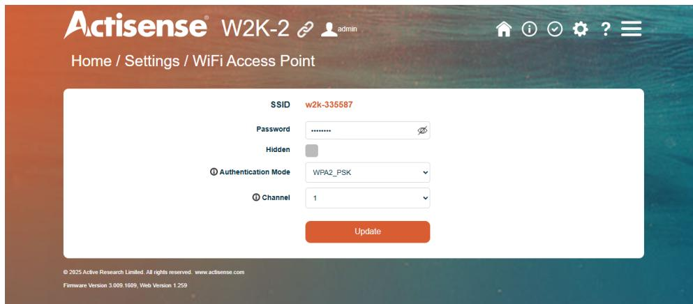
The authentication mode can be set by “Authmode”. By default this is “WPA2-PSK”, which is supported by most modern PCs and devices.
